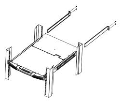
3. After the L brackets have been secured, tighten the front bracket screws.
